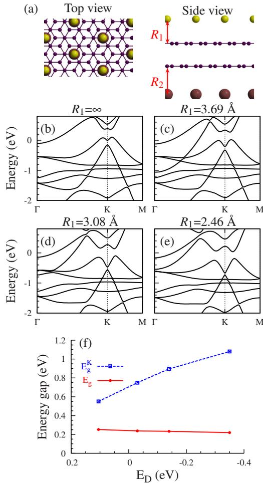
FIG. 3. (Color online) (a) The top and side views of the atomic structure of Na-adsorbed p-type bilayer graphene, where  $R_1$  ( $R_2$ ) is the distance between the Na (Pt) atoms and upper (lower) graphene layer, respectively. The electronic band structures of (b) the p-type bilayer graphene and [(c)–(e)] Na-adsorbed p-type bilayer graphene. (f) Changes in  $E_g$  and  $E_g^K$  as a function of a  $E_D$ .
