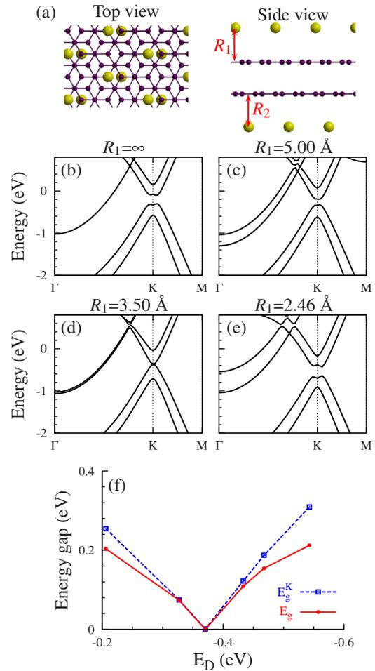
FIG. 2. (Color online) (a) The top and side views of the atomic structure of Na-adsorbed n-type bilayer graphene, where  $R_1$ ( $R_2$ ) is the distance between the Na atoms and upper (lower) graphene layer. The electronic band structures of (b) the n-type bilayer graphene and [(c)–(e)] Na-adsorbed n-type bilayer graphene. (f) Changes in  $E_g$  and  $E_g^K$  as a function of a  $E_D$ .
