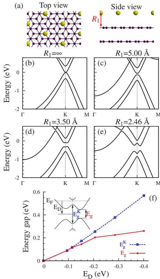
FIG. 1. (Color online) (a) The top and side views of the atomic structure of Na-adsorbed bilayer graphene, where  $R_1$  is the distance between the Na atoms and upper graphene layer. The electronic band structures of (b) the pristine bilayer graphene and [(c)–(e)] Na-adsorbed bilayer graphene. (f) Changes in  $E_g$  and  $E_g^K$  as a function of a  $E_D$ , where the schematic diagram of the electronic band structure of the bilayer graphene is in the inset.
