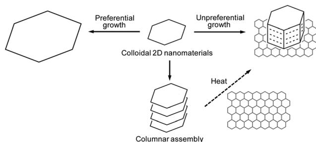
**Scheme 1** The formation of nanomaterials with a layered structure via columnar assembly and successive heating of colloidal nanoplates under argon.
