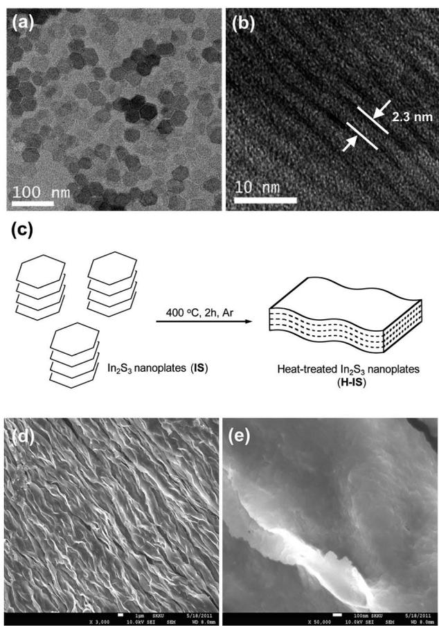
**Fig. 1** (a and b) TEM images of the colloidal  $\text{In}_2\text{S}_3$  nanoplates (**IS**), (c) cartoon of formation of a film-like big plate of  $\text{In}_2\text{S}_3$  (**H-IS**) via heating of columnarily assembled  $\text{In}_2\text{S}_3$  nanoplates and (d and e) their SEM images.
