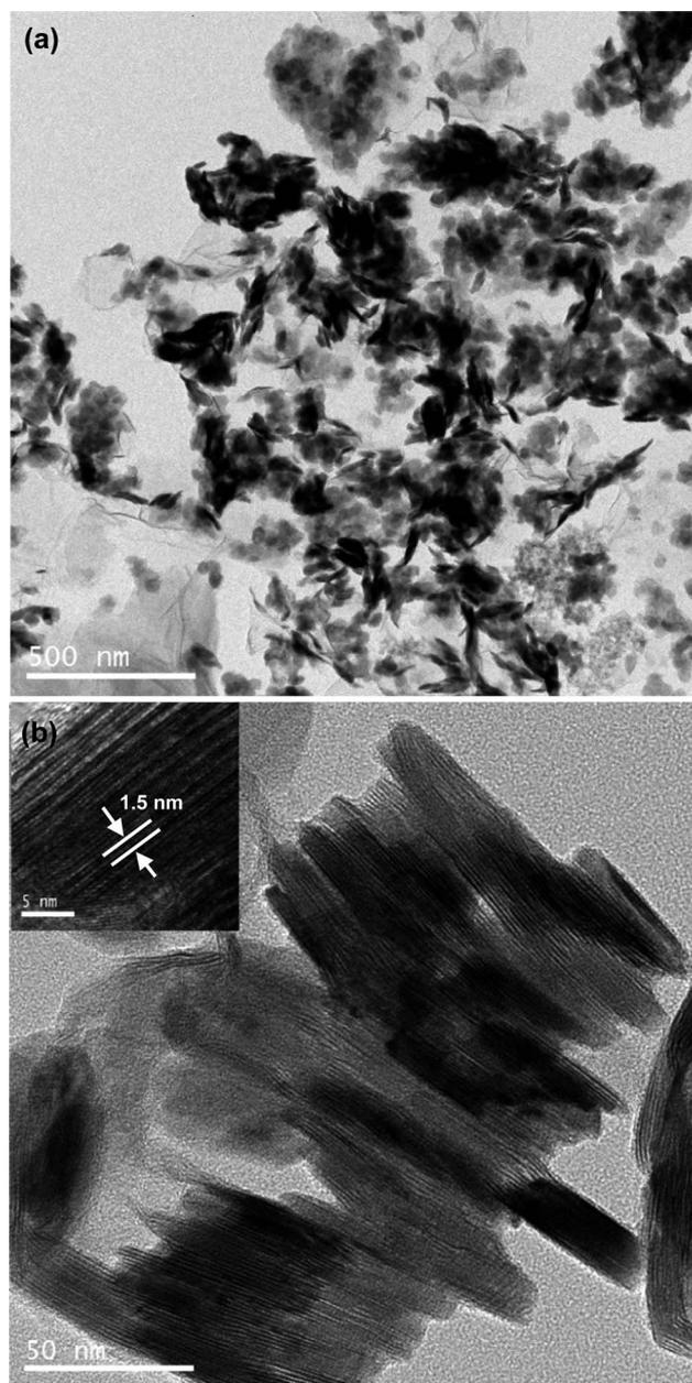
**Fig. 2** (a) TEM image of  $\text{In}_2\text{S}_3$  materials on graphene (**H-GIS-2**), prepared *via* the heating of columnarily assembled  $\text{In}_2\text{S}_3$  nanoplates in graphene and (b) their HR-TEM images.
