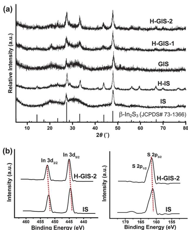
**Fig. 3** (a) Powder X-ray diffraction patterns of colloidal  $\text{In}_2\text{S}_3$  nanoparticles (**IS**), heat-treated  $\text{In}_2\text{S}_3$  nanoplates (**H-IS**), composites of graphene and  $\text{In}_2\text{S}_3$  nanoplates (**GIS**), heat-treated graphene composites of  $\text{In}_2\text{S}_3$  nanoplates (**H-GIS-1**, **H-GIS-2**) and (b) comparison of XPS spectra of **H-GIS-1** and **IS**.
