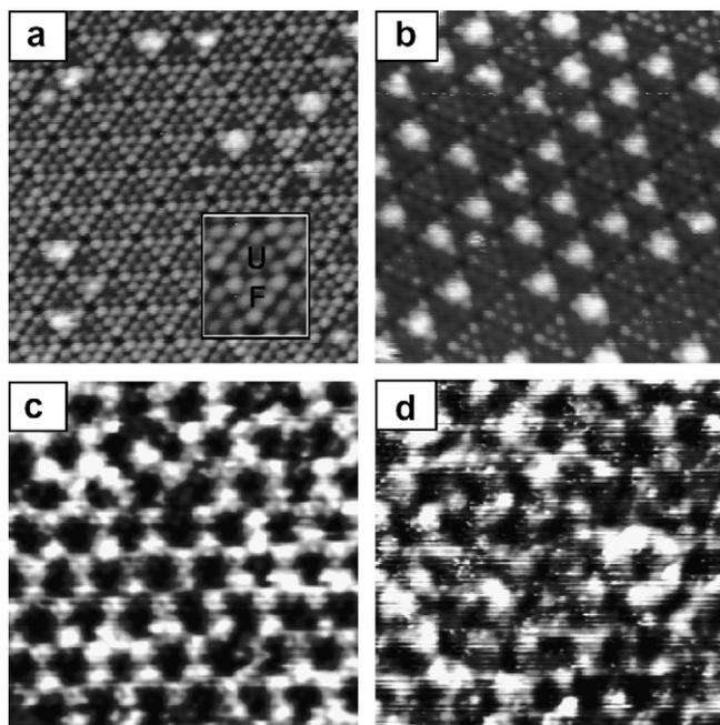
**Fig. 1.** STM images of the Na adsorbed Si(111)- $7 \times 7$  surface at RT with coverage (a) 0.04 ML, (b) 0.12 ML, (c) 0.22 ML, and (d) 0.33 ML. Faulted and unfaulted halves of a Si(111)- $7 \times 7$  unit cell are denoted by "F" and "U", respectively, in inset of (a). One finds that the sparse distribution of Na nanoclusters in (a) and (b) becomes a lattice-like array in (c).
