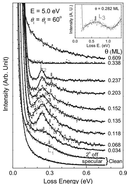
**Fig. 3.** Spectral change of HREELS spectra with increasing Na coverage  $\theta$ . The spectra have been measured with a primary electron energy of 5.0 eV at a specular geometry with incidence angle  $\theta_i = 60^\circ$ . The loss peak  $L_1$  and  $L_2$  attributed to an interband transition (marked by vertical bars) and a local atomic vibration, respectively (see text). Inset shows the spectrum at  $\theta = 0.282$  ML where a new loss peak  $L_3$  at 0.622 eV is apparent.
