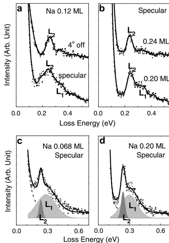
**Fig. 4.** Spectral changes measured at different scattering angles (a) and different coverages (b). The spectra at two different coverages have been fitted with two Gaussian peaks to find a broad ( $L_1$ ) and a narrow ( $L_2$ ) loss peaks in (c) and (d).
