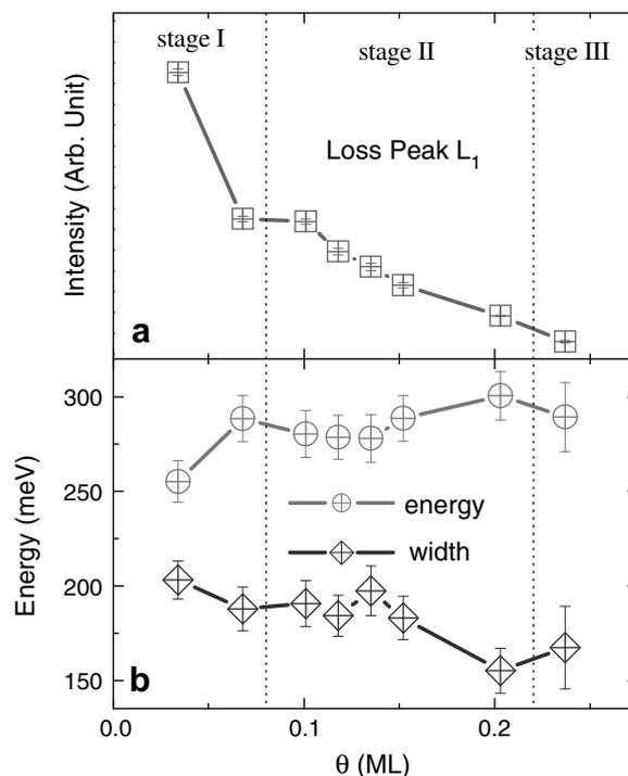
**Fig. 5.** Na coverage dependence of (a) intensity and (b) loss energy as well as the linewidth of  $L_1$ . One notices distinct behaviors for the two stages I and II of Na adsorption.
