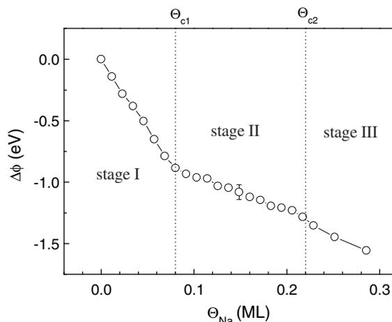
**Fig. 2.** Work function change ( $\Delta\phi$ ) versus Na coverage ( $\theta$ ). There are three distinct stages I, II, and III corresponding to gas-like phase, lattice-like phase, and decayed phase of nanoclusters, respectively, as suggested by a previous STM study (Ref. [7]).
